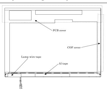
Figure 4-70 Replacing Samsung fluorescent lamp (WXGA) (1)
